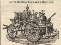
It is always ready to use instantly, and is m effective than a steam fire engine, because it is soon er brought into action and throws a powerful stream of water impregnated with carbonic acid gas for any
